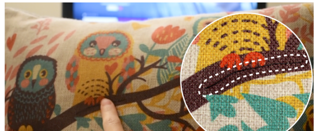
Figure 10 A user control the TV program using touch input on ThreadSense, hand-sewed on a cushion.
