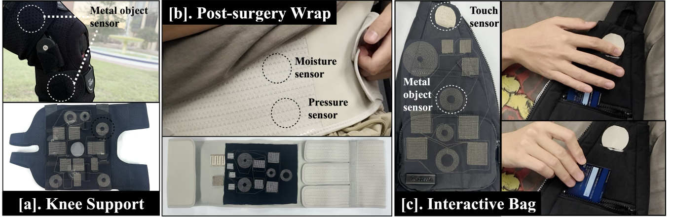
Figure 13: Three application examples created with Textro: (a) a smart knee support that detects slipping of metal reinforcements; (b) a post-surgery wrap for monitoring wound status and wrap pressure; and (c) an interactive bag for detecting user interactions.
