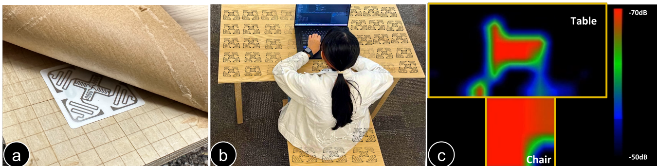
Figure 1: (a) Tagnoo is a computational plywood, consisting of a plywood panel augmented with a grid of RFID tags. (b) Tagnoo can be used to construct office furniture like a table and chair, which are capable of sensing the presence of an object or user. (c) The heatmap image of the RSSI values captured while a user is seated at a desk using a laptop. The upper segment shows the sensor data obtained from the desk, while the lower segment shows the sensor data obtained from the chair.
