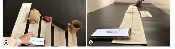
Figure 7: Near-field relays: (a) different transmission lines length and coil sizes; (b) multi-hop series connection.
