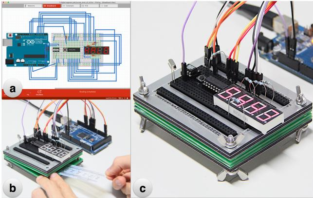
Figure 12. Revising the circuit. (a) Revising the breadboard schematic in Figure 10 by adding an RTC chip and a push button. (b) Loosening the four nuts and sliding new PCP into the circuit layer. (c) Results.
