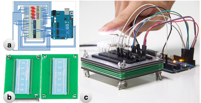
Figure 14. A demonstration for multi-layer PCP as a circuit becomes complex, incorporating eight pairs of a proximity sensor (photoresistor) and an LED controlled by two analog switches (MAX4617). The LED lights up as its paired photoresistor detects a nearby object. (a) Schematic. (b) Two pieces of generated PCP mounted on two circuit layers. (c) Result. Note that four PCBs are on the stack.
