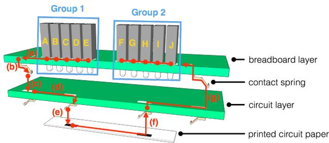
**Figure 5.** A simplified illustration of the CircuitStack mechanism shows the flow of electrical signals passing from (a) to (g) through routes and contact springs on PCBs, for establishing connections between the female headers of columns A to E and columns F to J.
