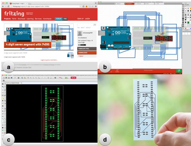
**Figure 10.** Converting a breadboard schematic into PCP. (a) Download a breadboard schematic from the Fritzing Project website. (b) Open the breadboard schematic with Fritzing software. (c) An EAGLE PCB file is created by first clicking on the *CircuitStack* button in Fritzing and (d) then on the *Autorouter* button in EAGLE to create the PCP result.
