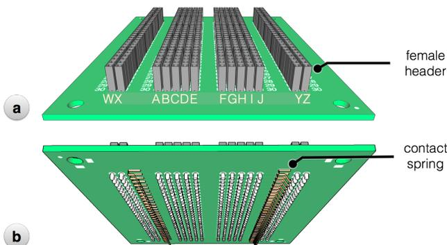
**Figure 6.** Breadboard Layer. (a) The top side is composed of  $14 \times 30$  female headers in which the columns are denoted as A to J and W to Z. (b) The bottom side is composed of two columns of contact springs, each with 32 rows, to deliver electrical signals across PCBs.
