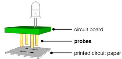
**Figure 3.** A conceptual illustration explains the technique of contact probes simultaneously reaching PCP conductive traces. The probes in our hardware system are actually contact springs for tolerating dimensional errors and ensuring connection reliability.
