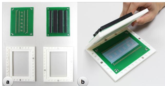
Figure 16. Magnetically-assembled CircuitStack. (a) Each 3D printed case fits one PCB layer. Magnets are on the edges of 3D printed case. (b) The conceptual assembled state of our magnetic-snapping approach.
