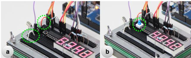
Figure 13. Using CircuitStack with manual wiring on the breadboard layer. (a) Swapping wires. (b) Replacing a push button.
