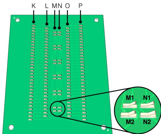
**Figure 8.** The bottom side of the circuit layer consists of six columns of spring contacts whose labels match that in Figure 7a. M1, M2, N1, and N2 are electrically shorted with columns W, X, Y, and Z (Figure 6a), respectively, when assembled. The pattern of M1, M2, N1, and N2 is repeated across columns M and N in this figure.
