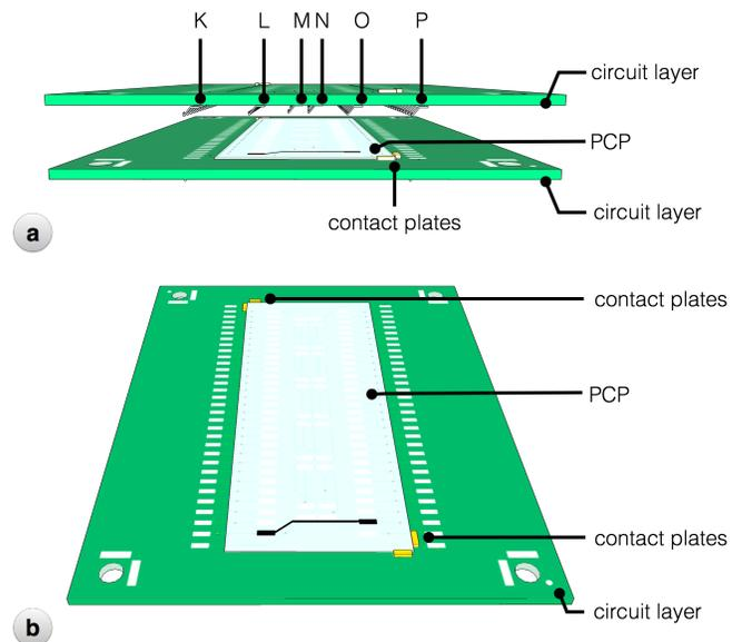
**Figure 7.** Circuit Layer. (a) The circuit layer consists of 6 columns (K to P) of contact springs on the bottom side. PCP is placed on the center of circuit layer. (b) The top side of circuit layer includes contact plates serving as physical constraints to aid PCP alignment. The translucency of PCP and marks on the top side help alignment as well.
