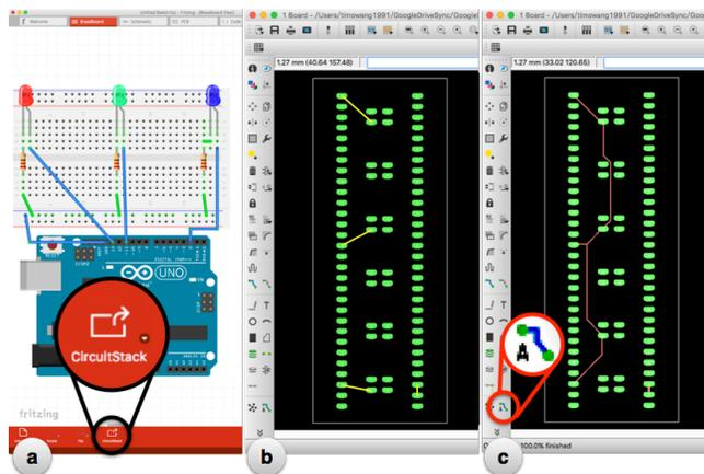
**Figure 9.** A breadboard schematic shown in (a) is displayed by the open source software Fritzing. A *CircuitStack* button is added to export the current breadboard schematic to an EAGLE file shown in (b) whose layout matches columns L to O in Figure 8. Clicking the enlarged bottom left button, *Autorouter*, instantly completes the wire routing in (c).
