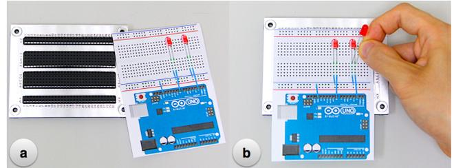
Figure 15. Printed breadboard schematic aids users to directly plug components onto the breadboard layer of CircuitStack.
