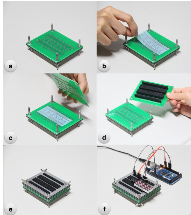
**Figure 11.** Step-by-step assembly process of using CircuitStack. (a) The assembly process begins with a circuit layer with four screws on the edges. (b) A piece of PCP is placed on the circuit layer. (c) Another circuit layer is placed on top of the PCP. (d) The breadboard layer is stacked upward. (e) An aluminum plastic panel support is placed on the top, and four nuts fastened the entire stack structure. (f) Electronic components and wires from Arduino are plugged and functioning.
