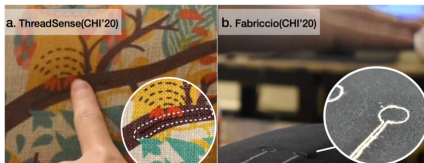
Fig 2 shows the smart textiles that can sense touch and midair gestural input to support explicit interactions. a) ThreadSense enables a single thread to locate user touches on the cushion. b) Fabriccio is a smart textile able to recognize midair gestures.
