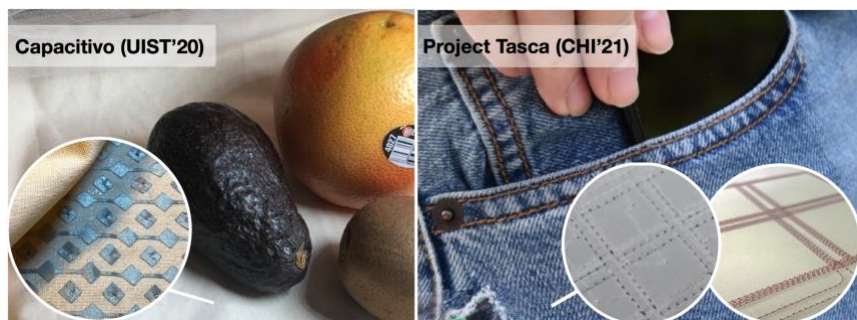
Fig 3 shows the smart textiles being aware of their contexts to support implicit interactions. a) Capacitivo is a smart textile able to recognize nonmetallic objects on it. b) Tasca is a pocket-based textile able to sense objects in a wearable pocket.
