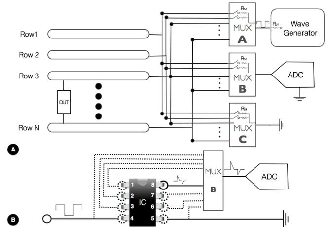
Figure 7. Hardware design for Component Recognition System (A) Each Row of Breadboard is connected to 3 multiplexers respectively for squared-wave input, data collection device and ground. (B) Multiplexer B switches between 8 pins of IC to retrieve waves passed to ADC.
