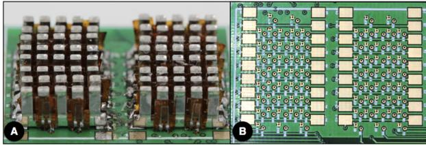
Figure 5. The sensing clips. (A) The lead wires of strain gauges were passed through holes on PCB and soldered on the copper pads next to the holes. Each pad was connected to a multiplexer cascading system, which transmitted the sensing value to our Pin Location Sensing system. (B) 8 \* 2 sets of sensing clips.
