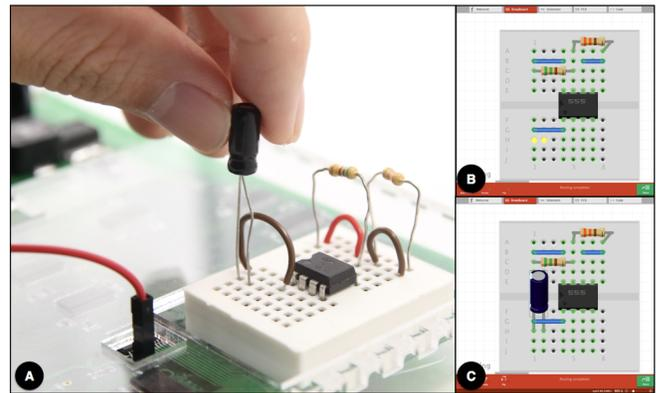
Figure 1. *CircuitSense* is a hardware+software system that facilitates automatic virtualization of physical circuit designs. (A) When developers place wires or electronic components on our *CircuitSense* breadboard, (B) Pin Location Sensing determines the location (highlighted in yellow) and the number of pins, followed by (C) Component Recognition identifying the type of that electronic component, and *CircuitSense* generates the corresponding software representation ultimately.
